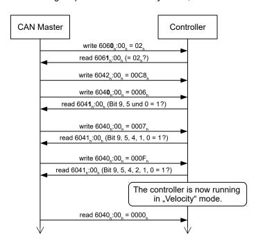
4. To stop the motor, set controlword (6040<sub>h</sub>) to "0".
