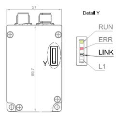
The green LINK LED is on if the EtherCAT cable is connected and flashes during data transfer.
