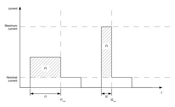
In the first section, t1, the current value is higher than the rated current. At time  $t1_{Lim}$ ,  $l^2t_{Lim}$  is reached and the current is limited to the rated current. A current that corresponds to the maximum current then occurs for a period of time t2. Hence, the value for  $l^2t_{l.im}$  is reached more quickly than in time t1.
